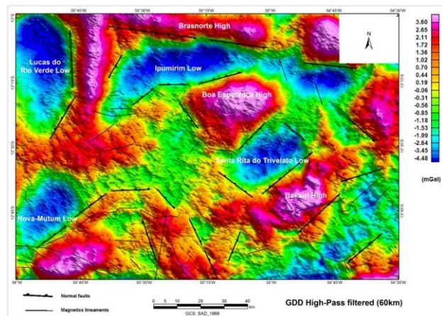
Figure 8 – Structural map of the study area over the High Pass filter of the Conformed gD (60 km).
