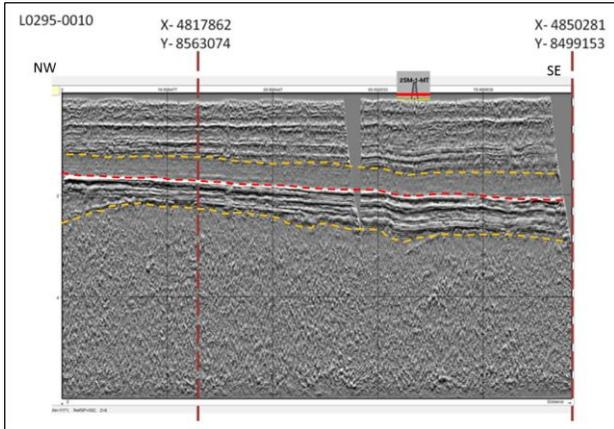
Figure 9 – Seismic Line L0295-0010 with a basic interpretation of the three main sedimentary layers.
