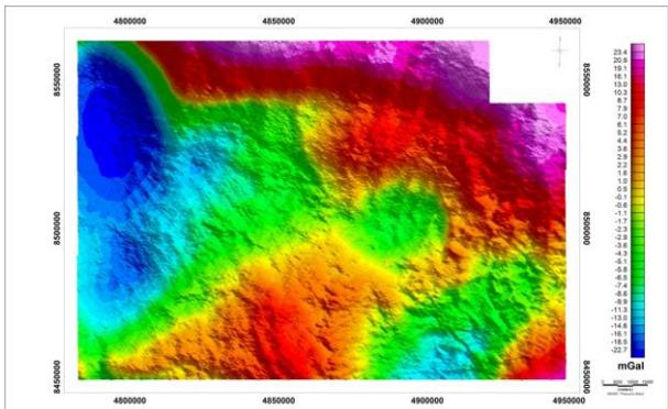
Figure 5 – Conformed gD - Terrain correction used: 2.5 g/cm<sup>3</sup>
