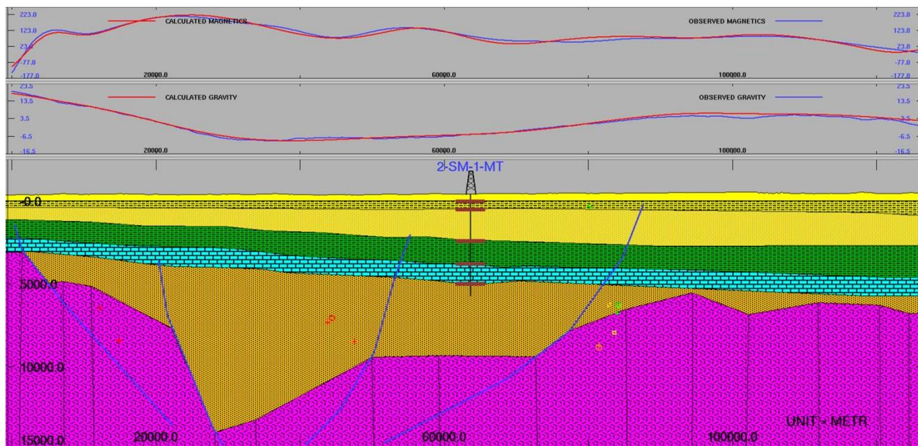
Figure 10 – Final model assuming basement interface locally reaches 13.000 meters of depth and using the density and susceptibility appointed in Table 1.
