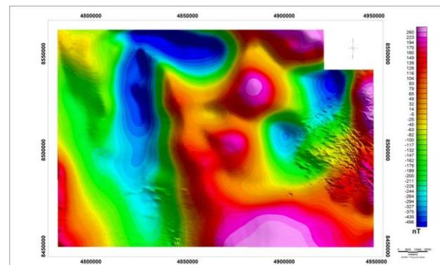
Figure 3 – Total Magnetic Intensity, IGRF removed and reduced to pole.
