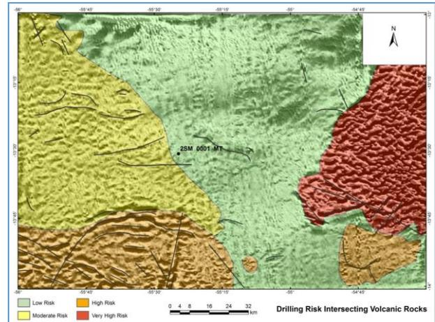
Figure 7 – Mached filter at 425 m of the Total magnetic intensity. The polygons represent the likelihood of wells intersecting igneous rocks in the area of study. The black lines represent mapped linear features in the filter.
